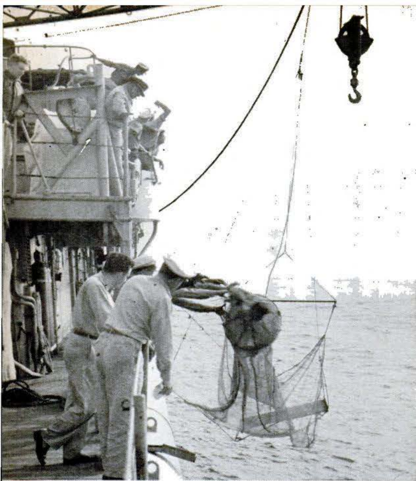
MID-WATER TRAWL , a conical 35-foot net with a 10-foot mouth, collects marine specimens. A new type will have electrically charged mouth to repel captured fish, prevent their escape.
